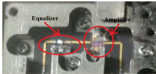
Fig-4 Developed single section amplifier with two section RL equalizer of IFM Receiver
