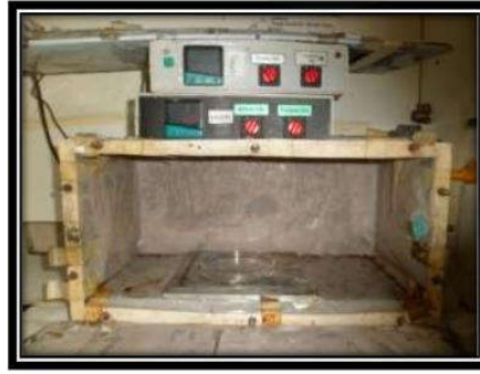
Fig.1b: The oven containing a qPVBCl Alkaline Anion Exchange Membrane
