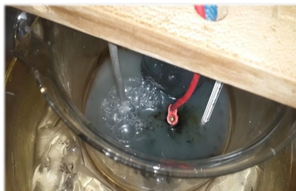
Figure 5: Shown bubbles formed around the electrodes
